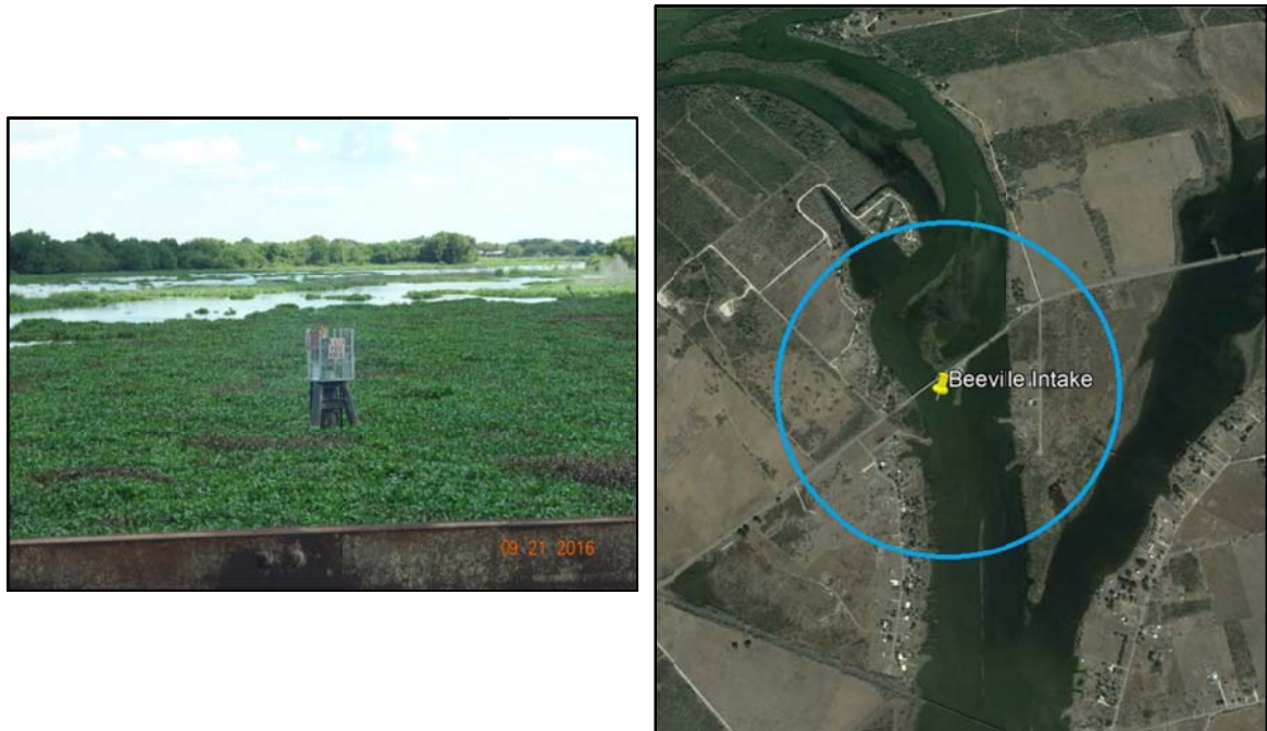
Figure 6. Hyacinth Surrounding the City of Beeville’s Intake Structure (left) and Buffer Zone (right)
